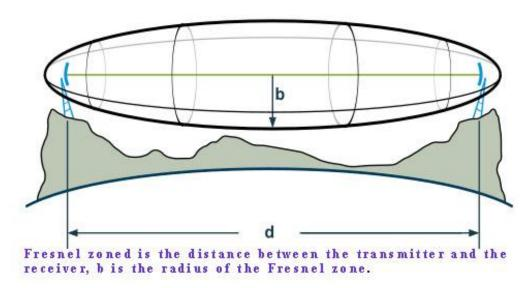
The max diameter of the Fresnel zone corresponds to the max height and width of the Capture Zone. The Capture Zone is the area the receiving antennas has to be in to receive the signal. Very useful when building arrays or using multiple antennas for MIMO.
