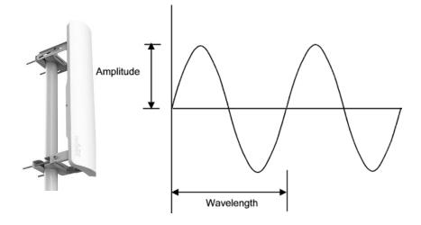
The near field is 1 wavelength away from the antenna The transition zone is the  $2^{nd}$  wavelength The  $3^{rd}$  wavelength and farther is the far field
